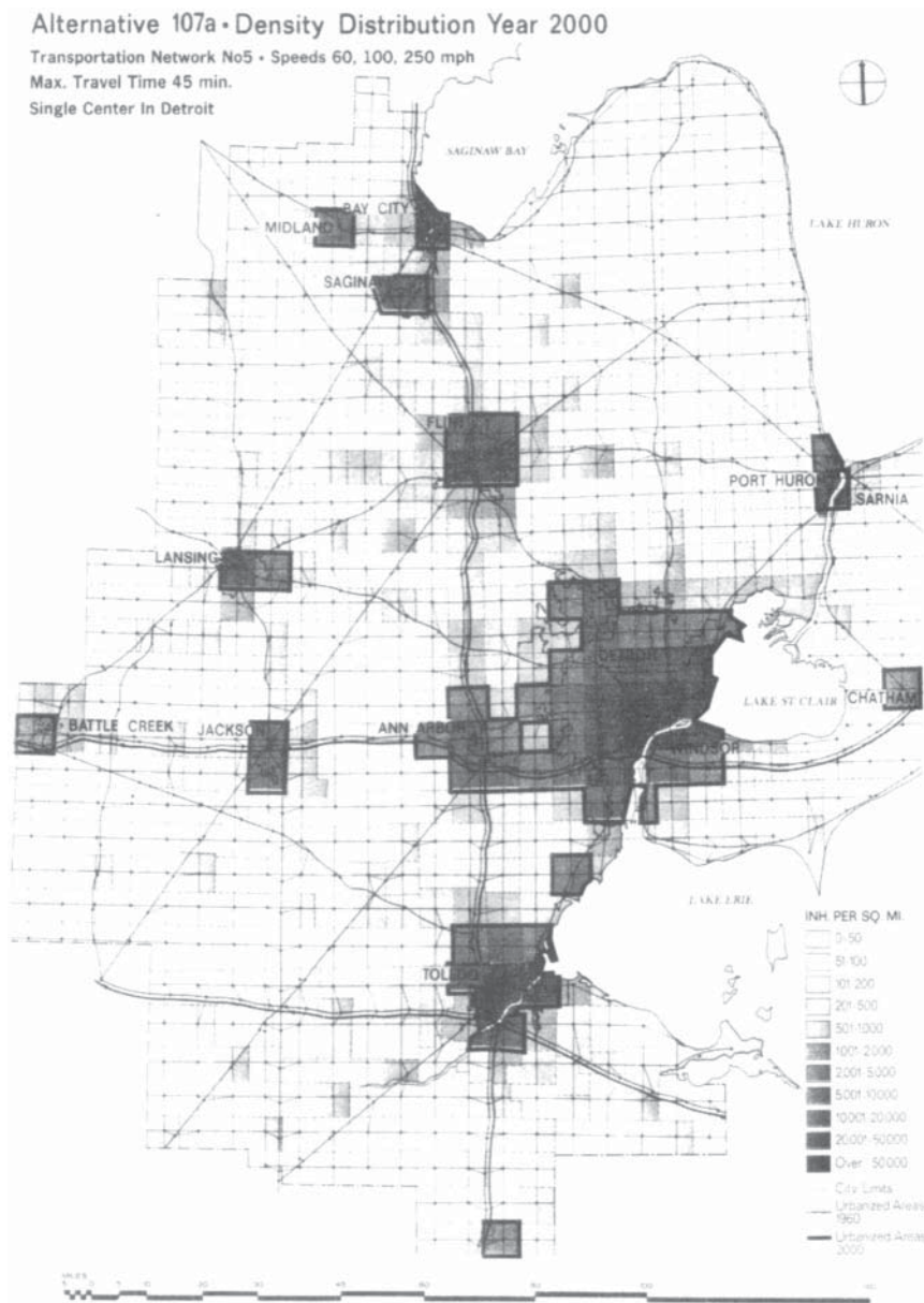
Fig. 14. Project for the urban Detroit area: Alternative of population densities based on 45-minute travel time and three projected transportation speeds.
